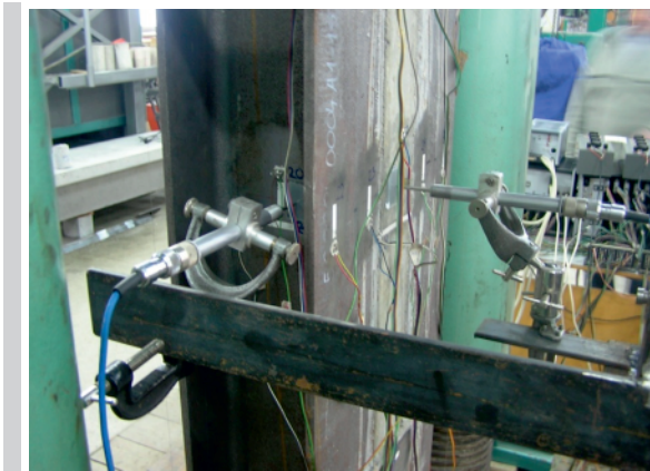
Figure 2. Location of gauges on the middle part of the tested column
