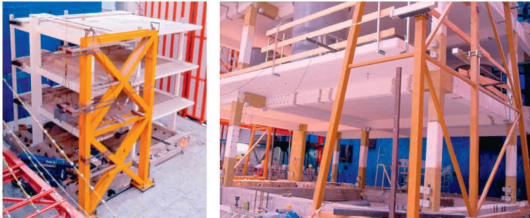
Figure 2. SPEAR test structure frame: (left) un-retrofitted, (right) retrofitted with FRP jackets
